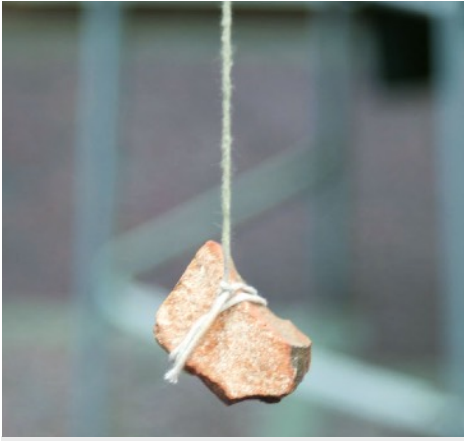
Improved plumb line with a string and a stone.
